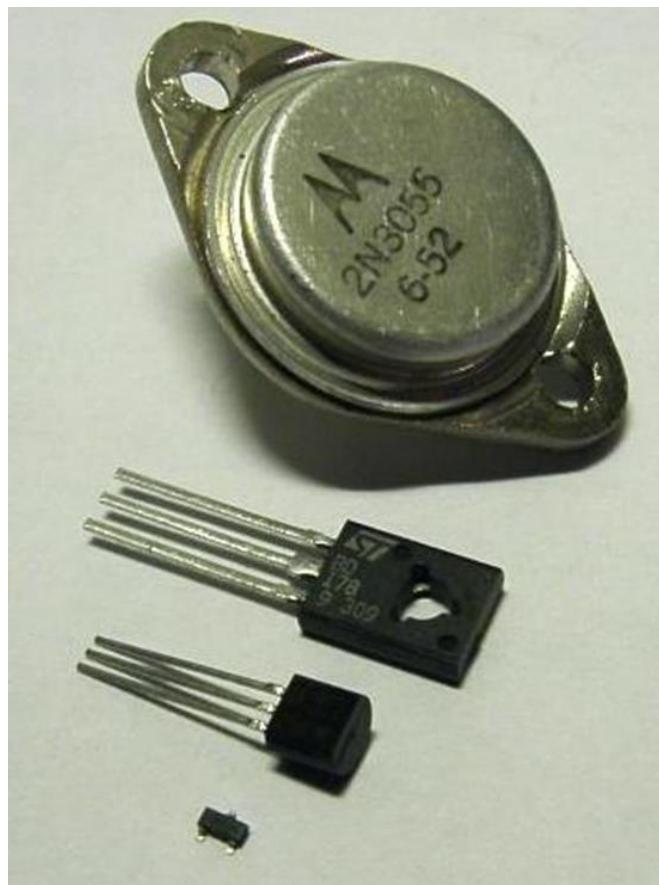
**Slika 8: Primeri tranzistorjev**Vir: [http://en.wikipedia.org/wiki/File:Transistorer\\_\(cropped\).jpg](http://en.wikipedia.org/wiki/File:Transistorer_(cropped).jpg)
