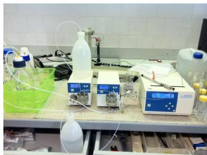
Slika 9: Instrument HPLC (foto: Centrih, T., 2014)
