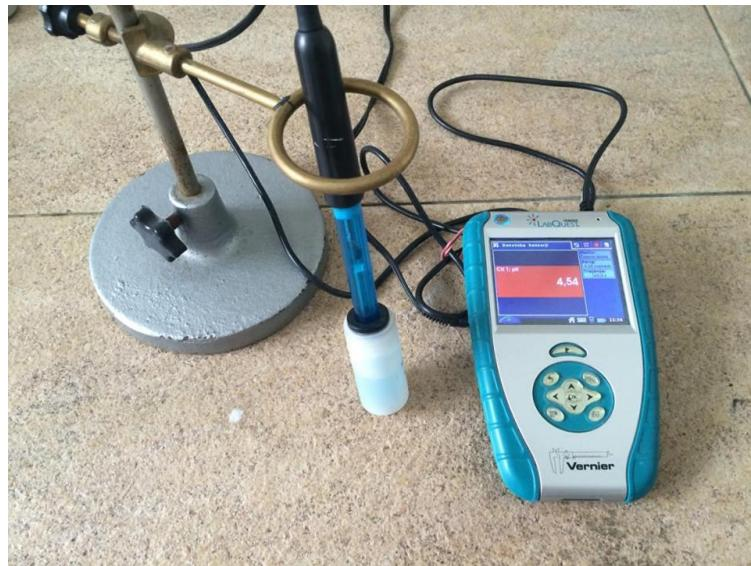
Slika 15: Merilnik pH in vmesnik LabQuest Vernier
