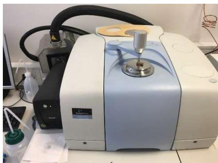
Slika 23: IR-spektrometer
