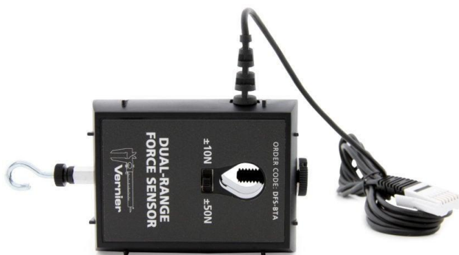
Slika 13: Digitalni silomer Vernier ( https://rb.gy/jba86 )
