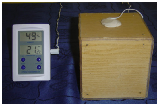
Slika 2: Merilna kocka (stranica 10cm) in merilnik temperature
