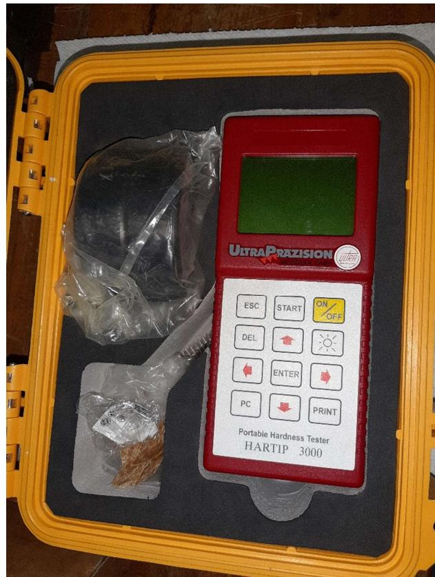
Slika 24: ULTRA PRAZISION- PORTABLE HARDNESS TESTER- HARTIP 3000
